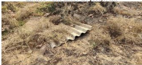
ACM left near the Overhead Water Tank
